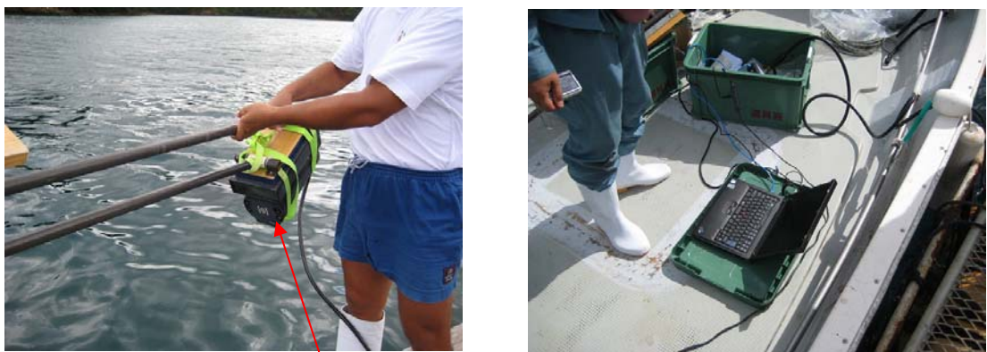
Figure 2. Attaching the DIDSON to the plastics pipe (left), control computer and battery unit onboard support boat (right).
