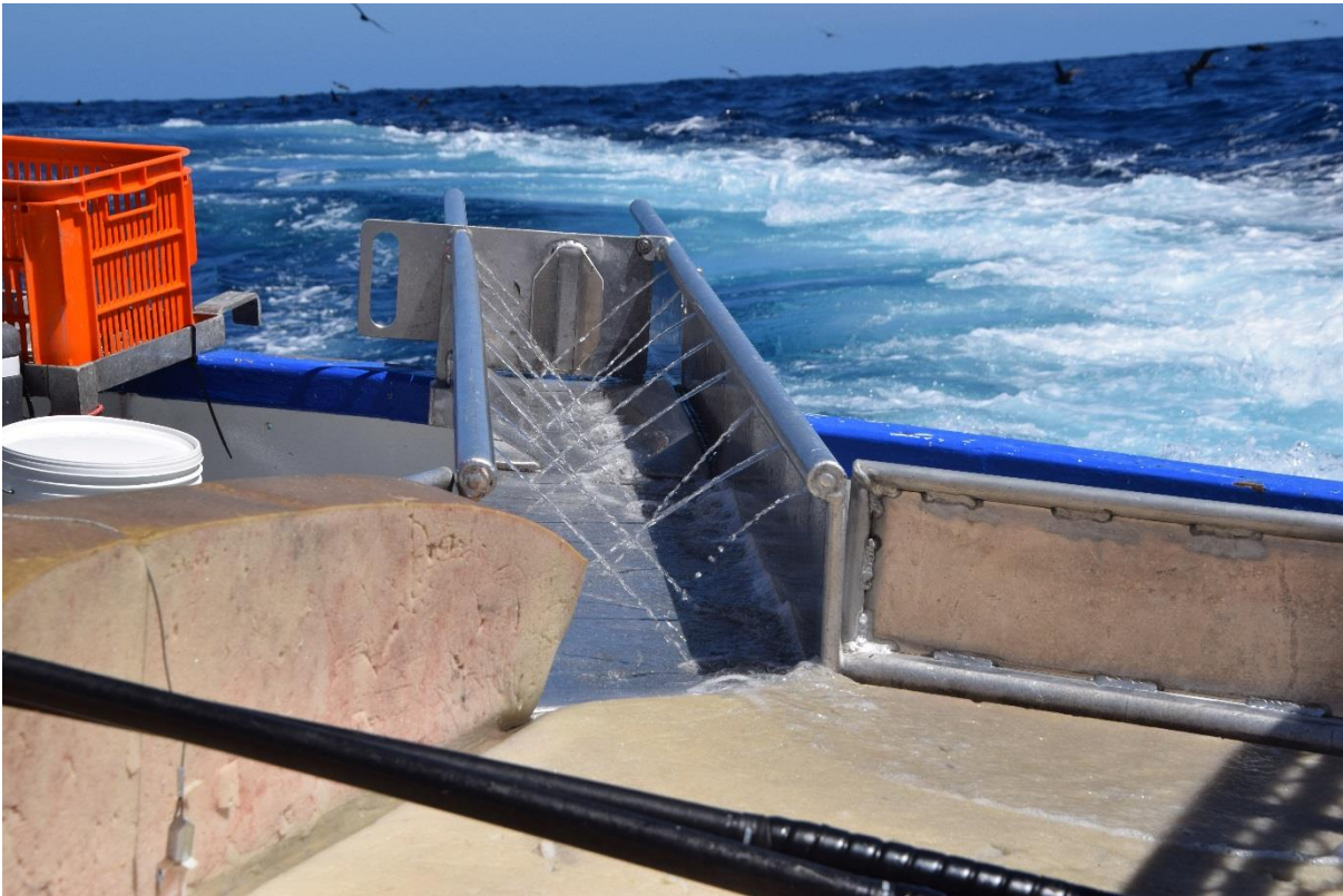
Figure 2: Redesigned fish chute with water jets running.
