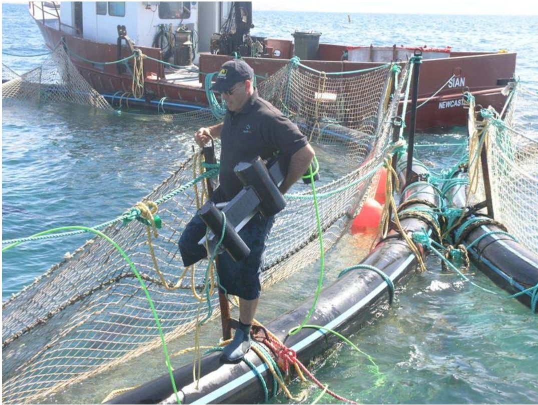
Fig. 8. GigE stereo-video camera being retrieved from the transfer gate
