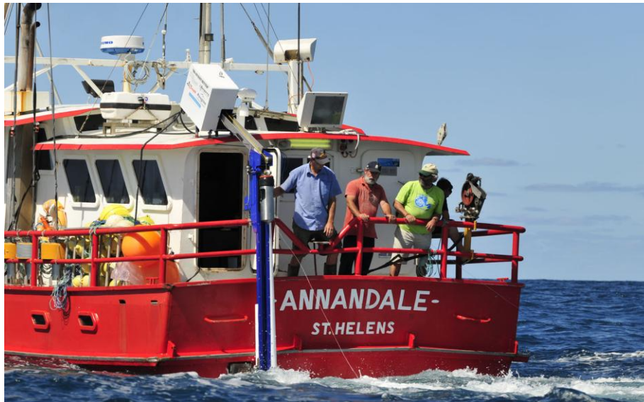
Figure 1. The underwater setting machine being trialled off eastern Australian in January 2010. The hydraulics and control box are mounted on the roof to reduce the number of pulleys involved in connecting the hydraulic motors to the capsule. Fewer pulleys increase the transfer of energy from hydraulic motors to the capsule, which increases depths attained for a given cycle time.
