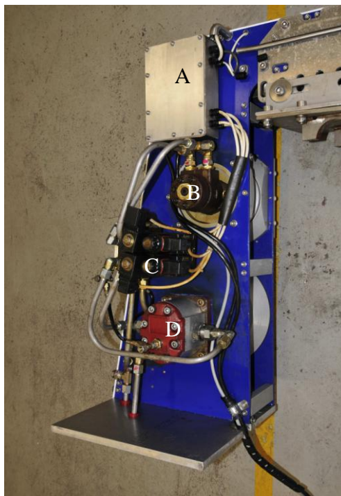
Figure 2. The drive system of the underwater setter. Shown are the control box (houses the PLC, data recorder and GPS; A), recovery motor (B), solenoid and relays (C) and pull-down motor (D). The on/off button and brake and timer are on the other side. The pulleys holding the spectra rope are barely visible beneath the hydraulic motors.
