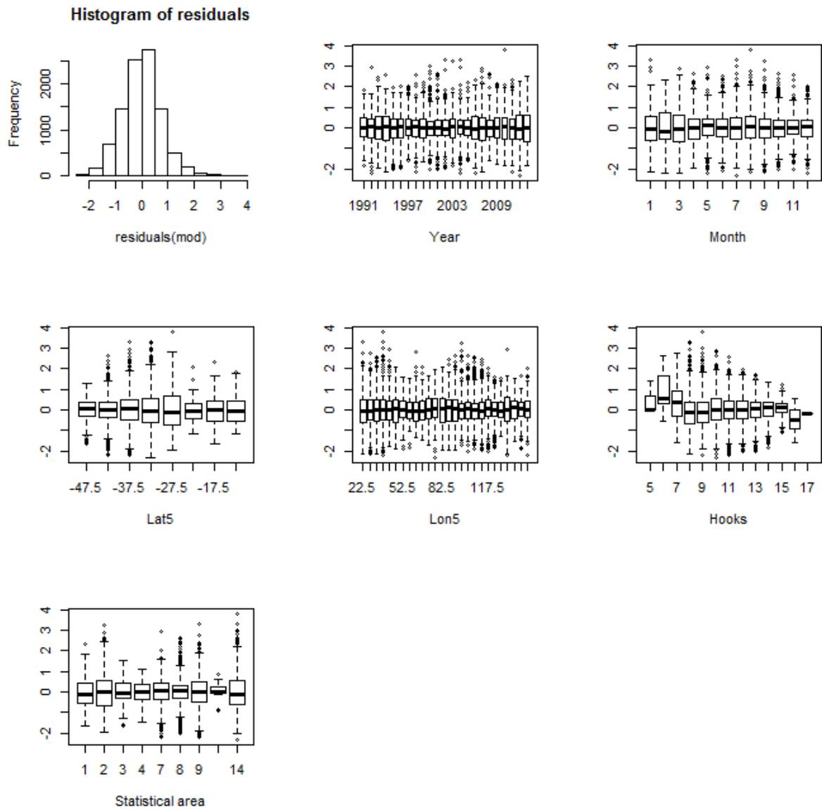
Figure 22: Histograms of residuals and boxplots of residuals versus covariates for the Indian Ocean positive GLM. Lat5 and Lon5 represent the latitude and longitude in 5 degree categories. Hooks have been categorized by taking the natural logarithm and grouping by unit on the log scale.
