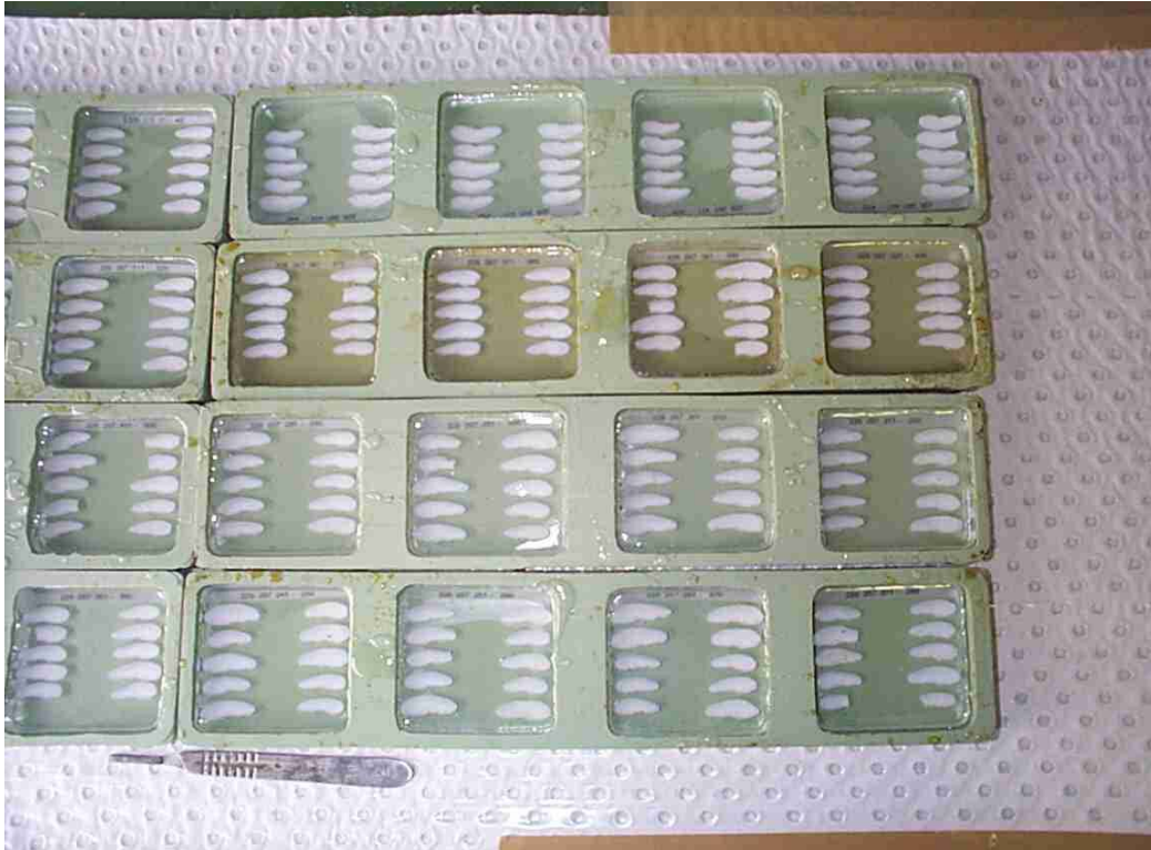
1. Silicone moulds used to embed otoliths in polyester resin. Source: Kyne Krusic-Golub, Central Ageing Facility, Australia.
