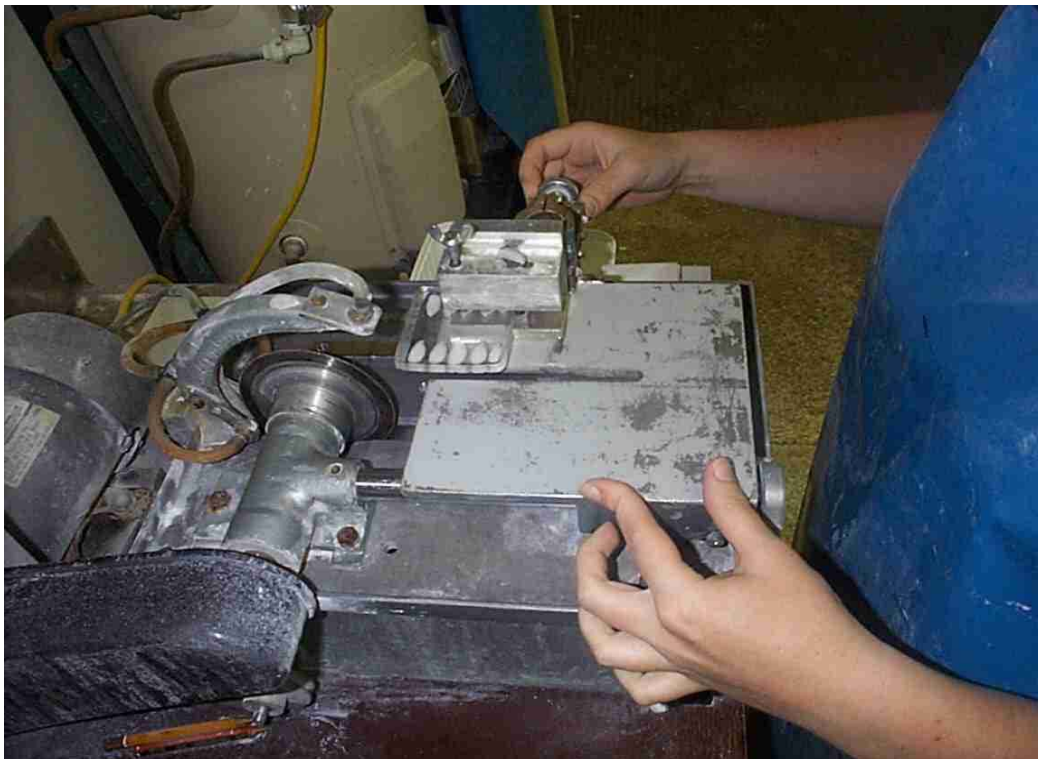
2. Modified Gemasta™ sectioning saw in use. Source: Kyne Krusic-Golub, Central Ageing Facility, Australia.
