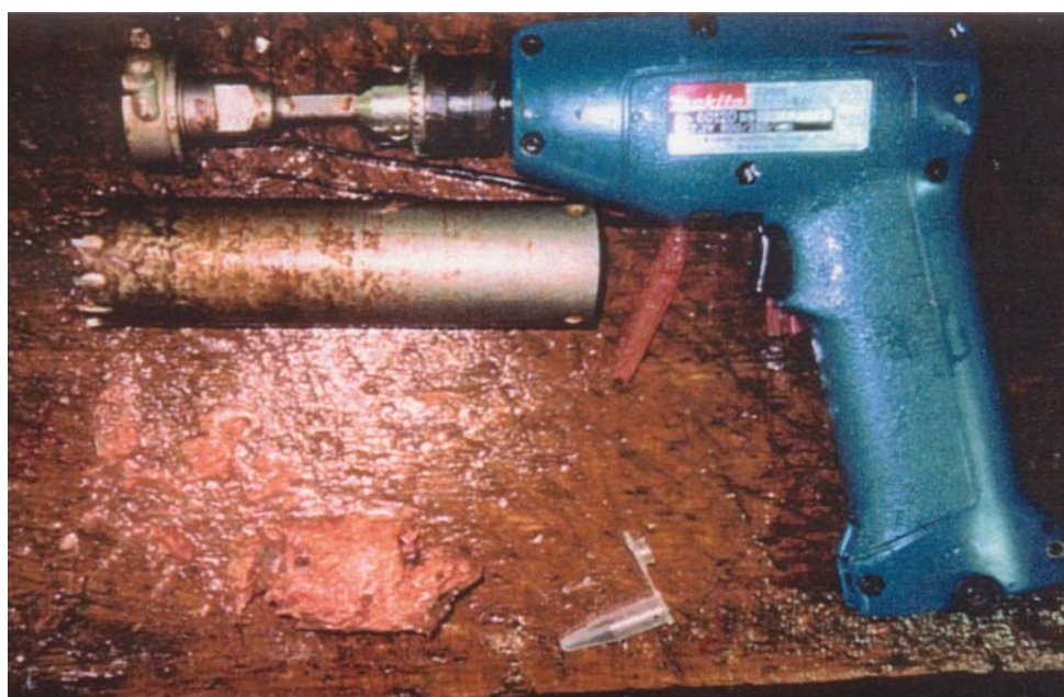
Figure 4.4 Battery-powered drills can be used for extracting cores from un-frozen fish (figures were provided by CSIRO, Australia and NRIFS, Japan).
