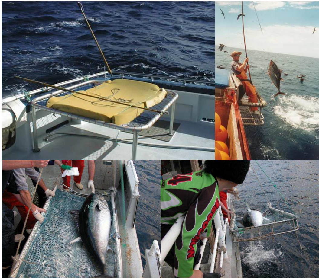
Figure 6.4. Fish landing techniques. Upper. Landing of poled fish in the Great Australia Bight onto a tagging table. Lower. Landing of southern bluefin tuna from a longline vessel using a lifting cradle. Pictures by Thor Carter. C:\Data\Alistair\Pictures and Images\Fish Tuna Pictures
