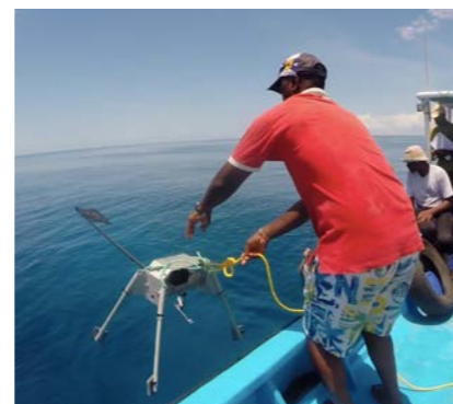
Fig 7: Deploying a BRUVS. (Source: Cordio East Africa-watch)
