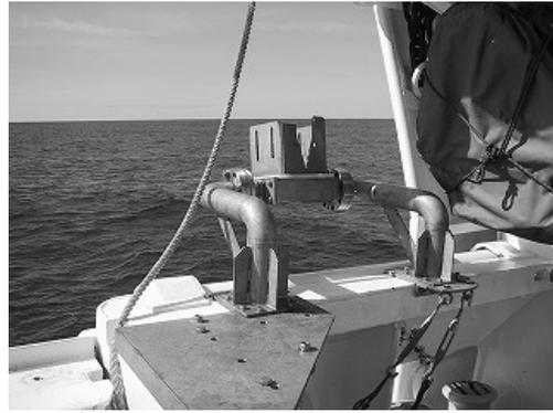
**Photo 4** Mount of underwater setting device.
