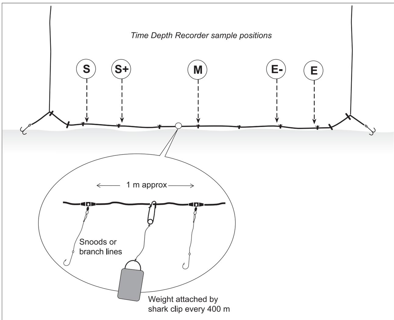
Figure 7. Sampling positions on the longline.
