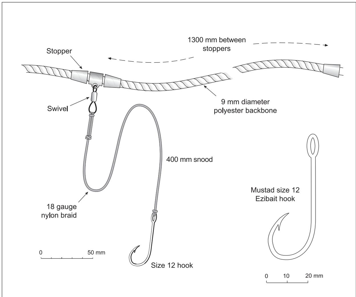
Figure 3. Detail of a section of autoline longline gear.
