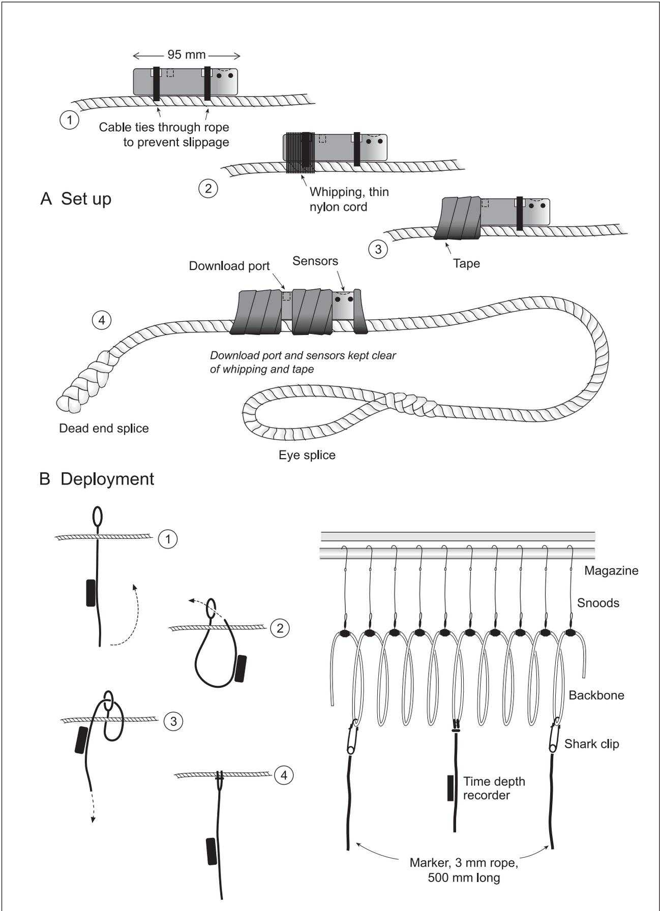
Figure 6. Time Depth Recorder: A—as set up; and B—as deployed on the longline.
