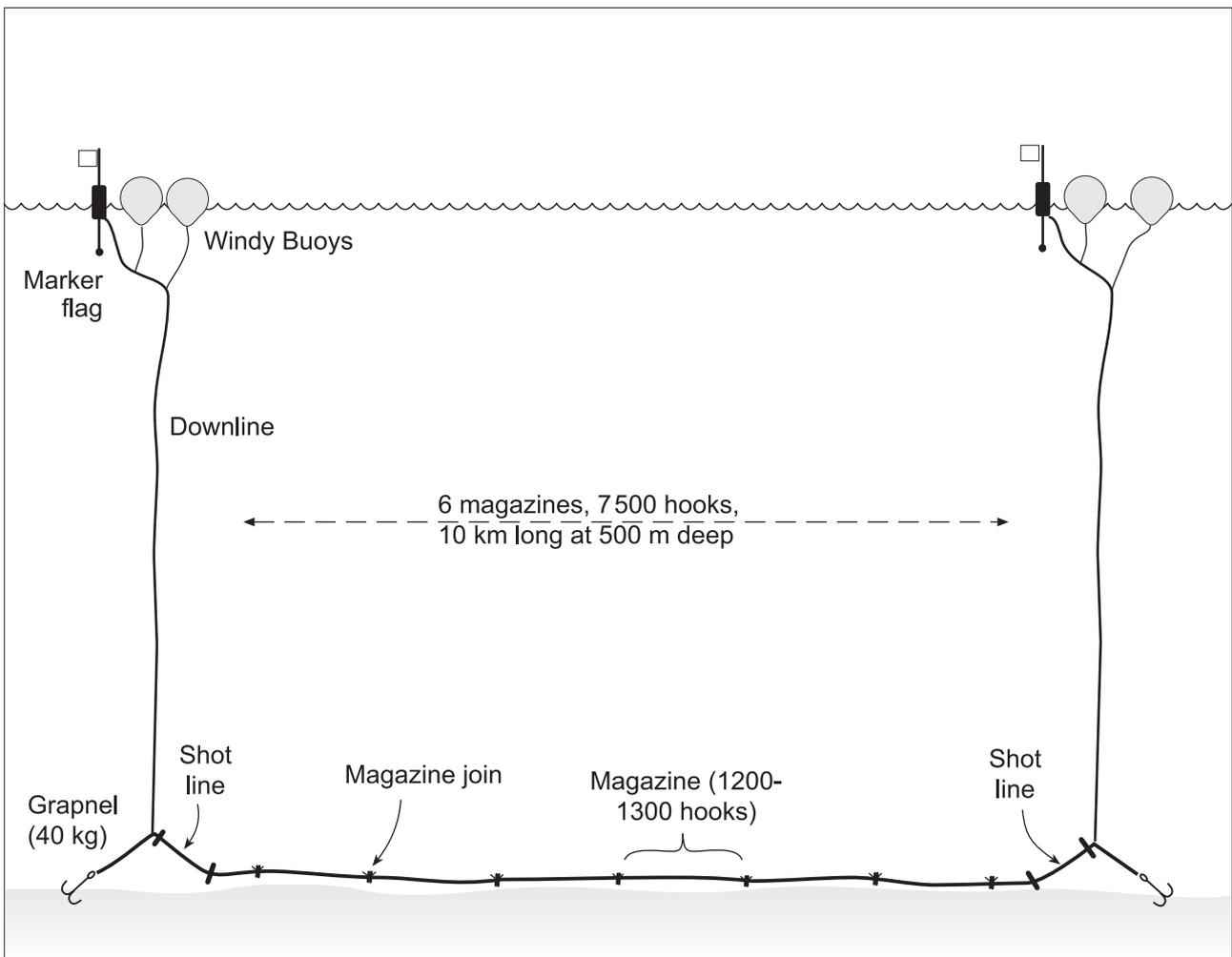
Figure 2. Diagram of a typical demersal longline.
