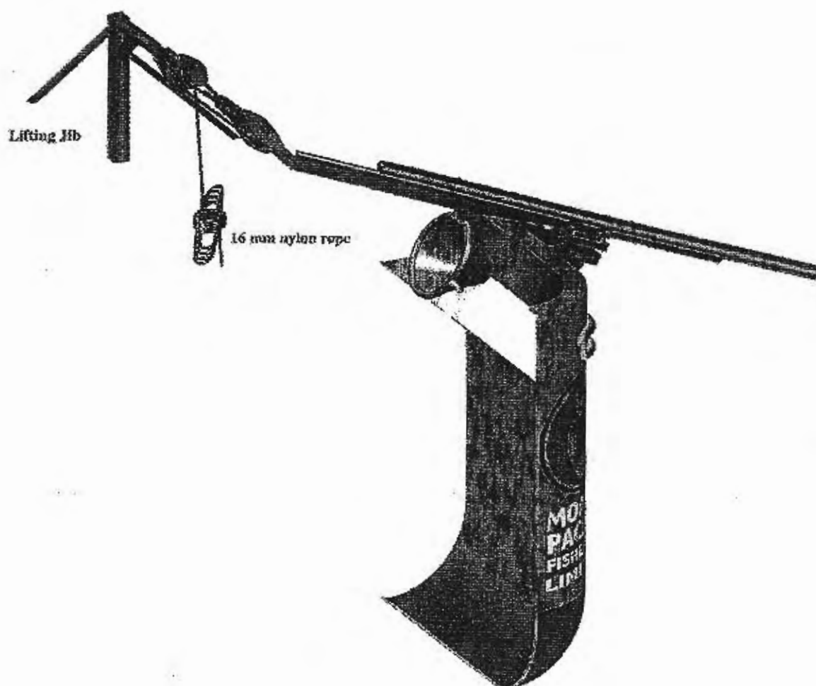
FIGURE 16. SECOND METHOD OF DEPLOYMENT AND RECOVERY OF THE CHUTE TRIALED ON F.V. ATU S.
