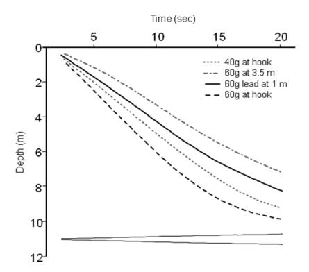
Figure 2. Average sink profiles of the two weighting regimes compared in the trial and two additional regimes with potential relevance to the fishery. The 95 % confidence bounds are shown as horizontal bars at the bottom of the figure. If the difference between any two average
