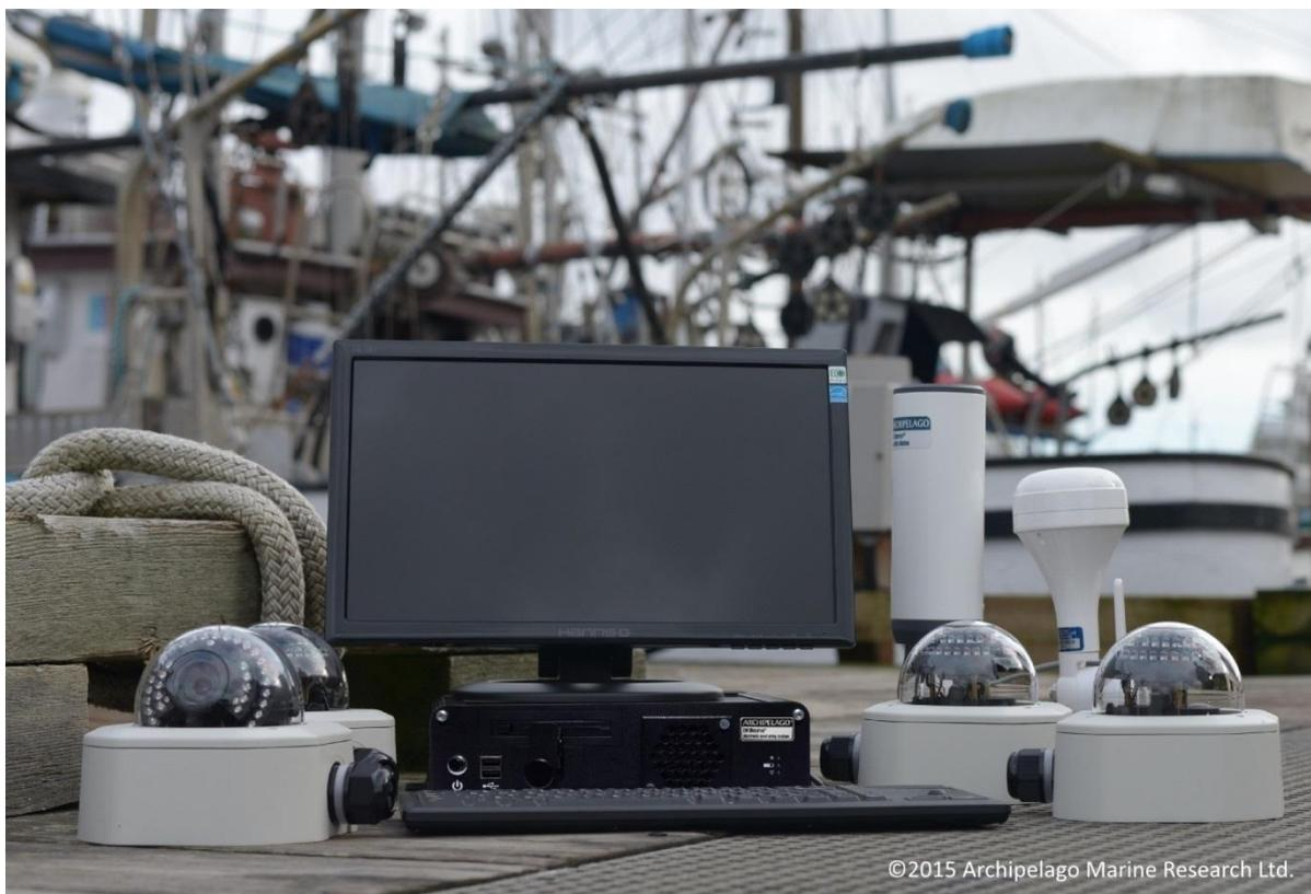
*Figure 1. A typical e-monitoring system which includes cameras, sensors and a computer modem to detect and record fishing activity. ( Photo: Archipelago Marine Research Ltd)*
