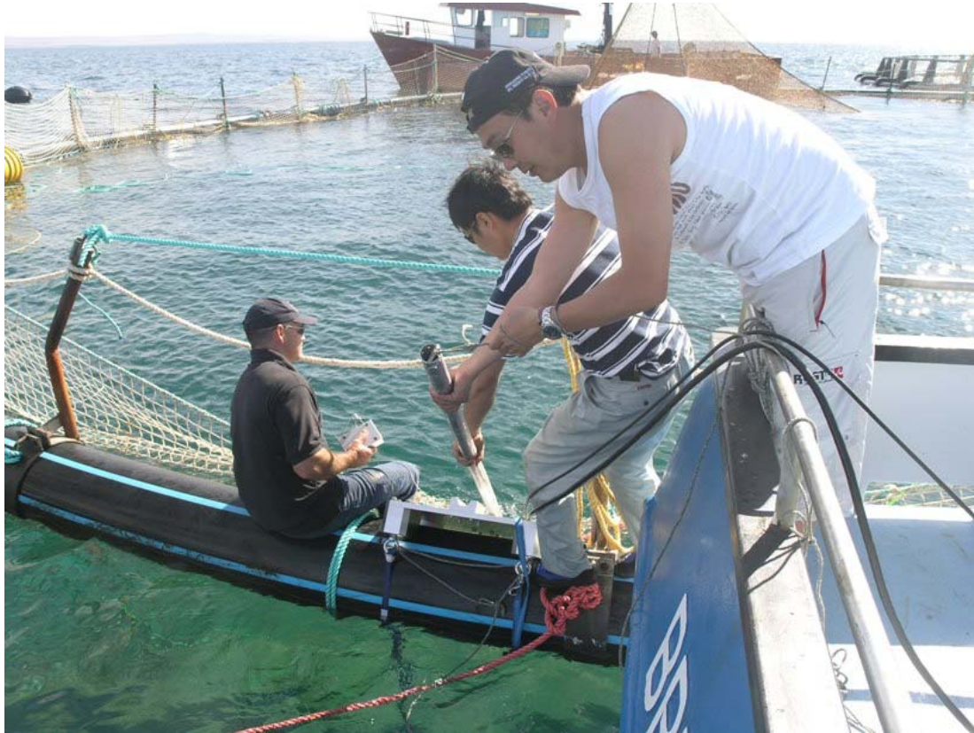
Fig. 9. Mounting the DIDSON sonar module and adjustable arm on the collar of the research pontoon
