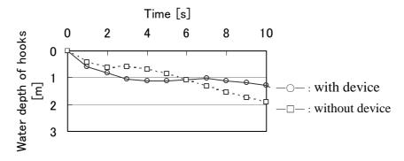
Figure 3 Comparison of the average water depth with and without the device.
