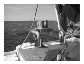
Photo 4 Mount of underwater setting device.
