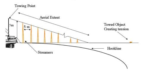
Figure 1. Diagram of Bird Scaring Streamer Line.
